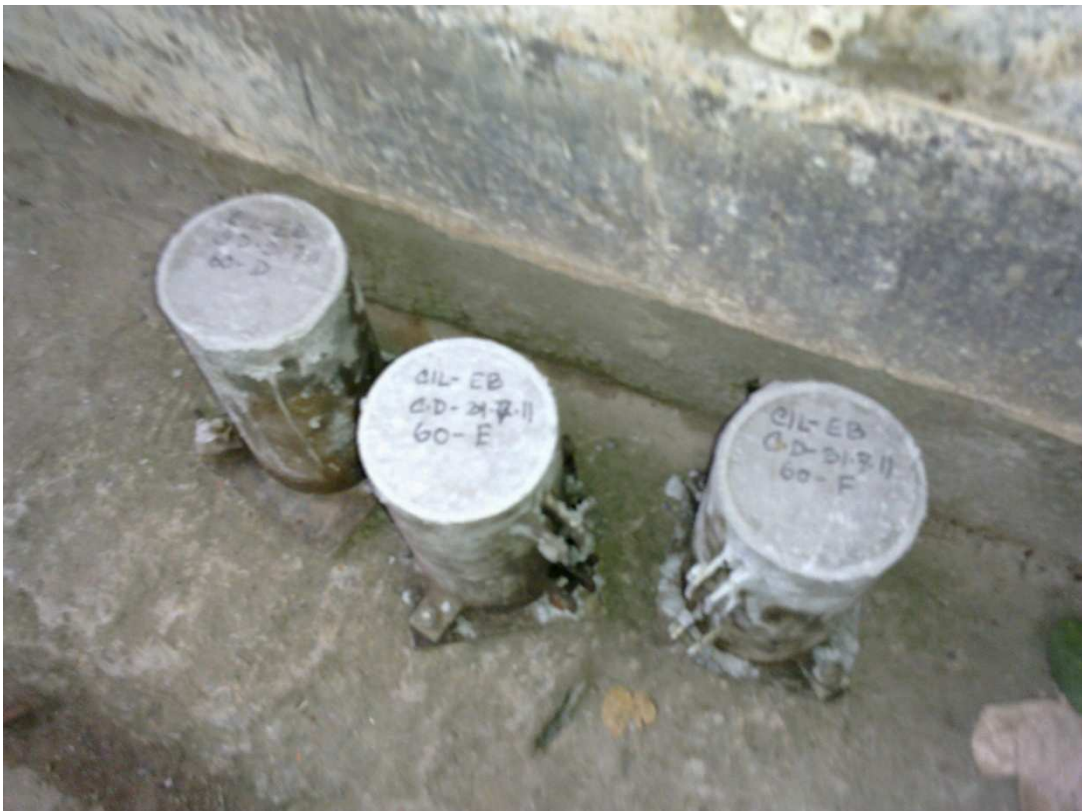
Concrete cylinder is taken for actual concrete strength test
